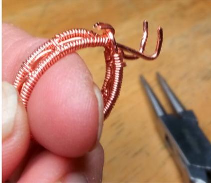
Put your ring back on the mandrel and push it down. Remove it, flip it over and put the ring back on the mandrel to keep the shape uniformed. This also helps to work harden the wire.
