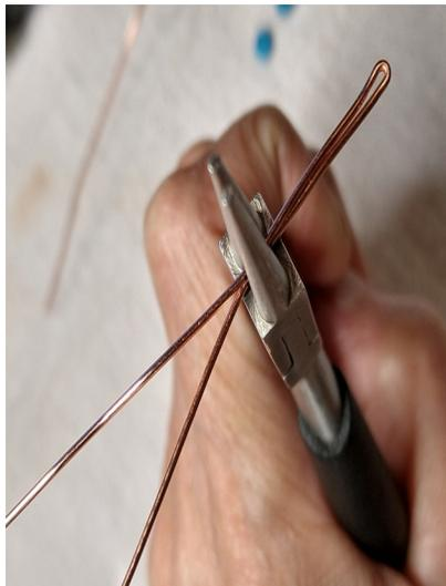
Using needle nose pliers, hold the frame at the inch mark. Make sure the wire is placed at the bottom of the pliers as seen. Then bend the wire around the pliers so they are straight with the folded part, as seen
