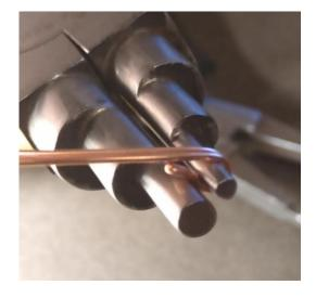
Place your pliers between the wires. Grip about ¼ inch below the hook and bend the wire outwards
